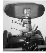
Side adjustment: After loosening the screws (3) the headrest can be pushed sideways. Tighten screws again (see the page on torque).
