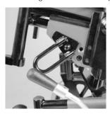
Position of the front wheelchair tie down restraint and the tie down label The position is the same for both the self-propelling and the attendant push wheelchairs.
